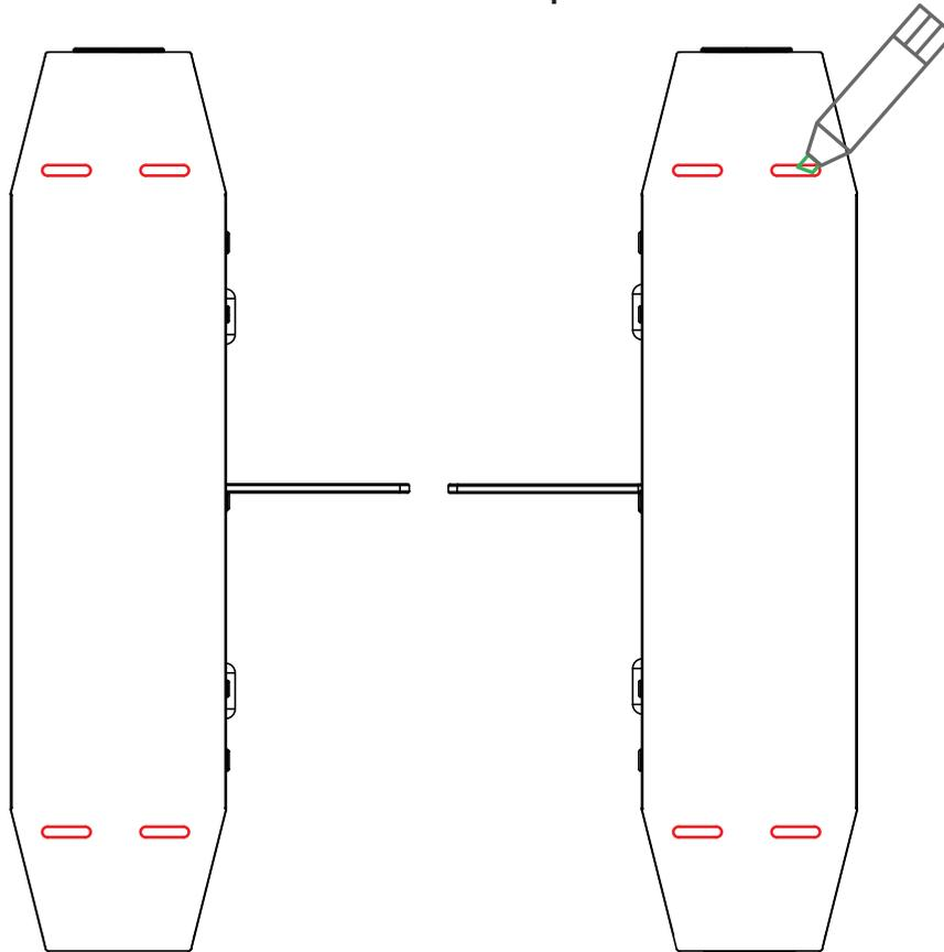
Move the device away and embed M12 \* 100 expansion screws according to the marked hole positions
