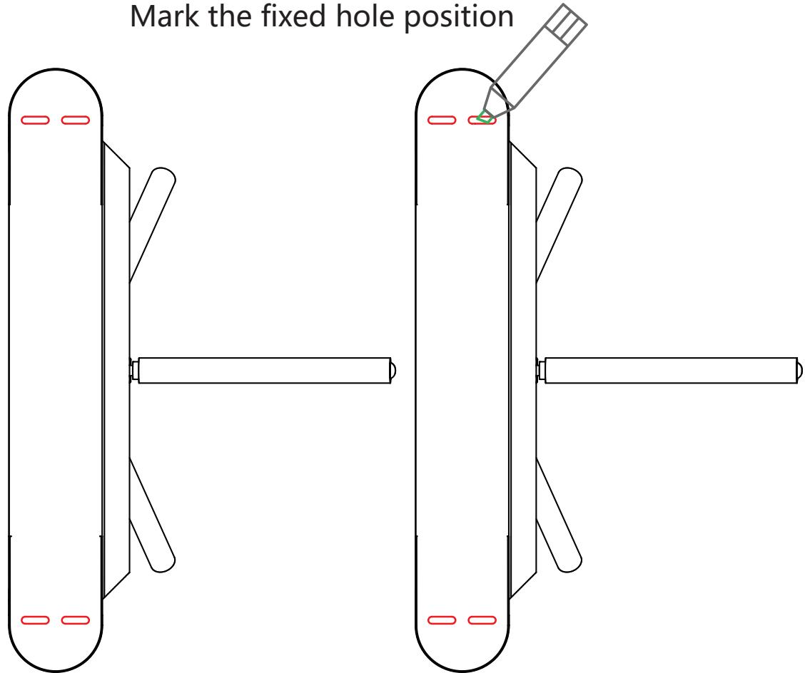
Move the device away and embed M12 \* 100 expansion screws according to the marked hole positions
